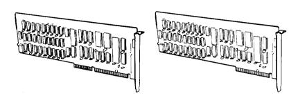
Usually it does not matter which slot an option card occupies as long as the card fits in the slot. For example, you can place some 8-bit cards in a 16-bit slot. However, you must follow these guidelines when deciding which slot to use:
